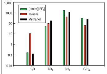
Figure 2 Comparison of the Henry's law constants for H2O, CO2,  $CH_4$  and  $C_2H_6$  in [bmim][PF<sub>6</sub>], toluene and methanol at
